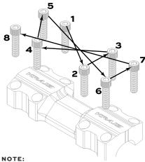
Make sure each bolt has been screwed in evenly before tightening.
