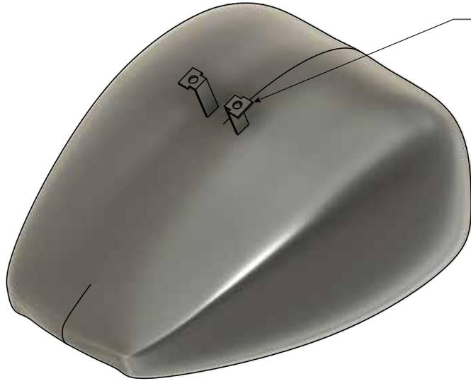
The upper portion of original gauge bucket mounts must be shortened.
