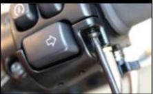
Open switch housing to allow access to throttle tube.
