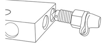
**NOTE:** Plug bleeder is intended for single disc bikes. Remove if bike has twin discs.
