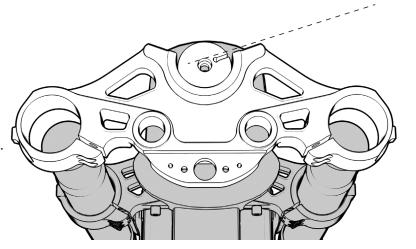
**NOTE:** If the forks & wheel were removed prior they can be installed after top tree is installed.
