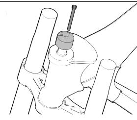
With slit aligned, torque yoke nut to procedure.
